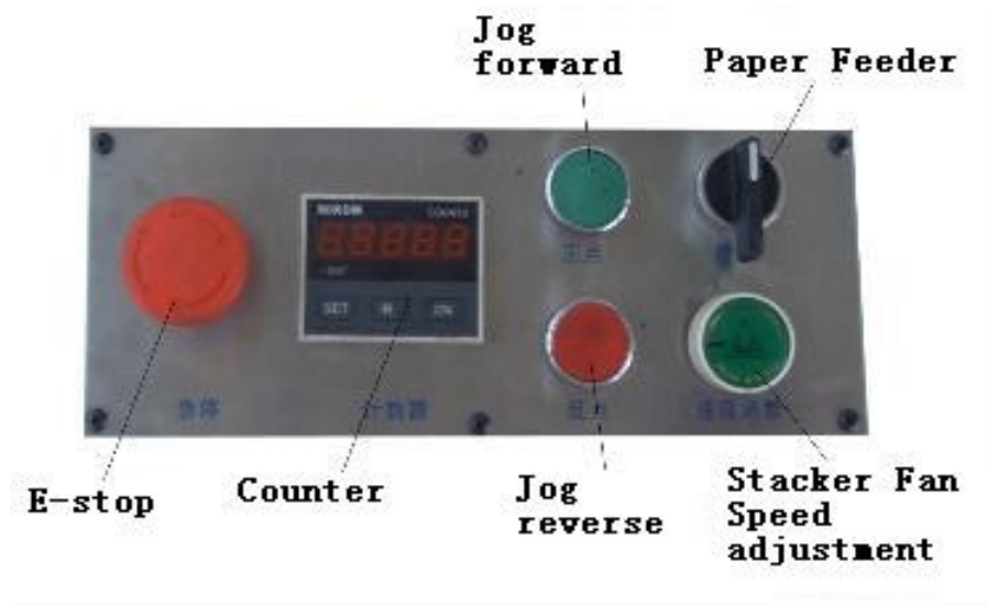
Paper Stacker Control Panel
