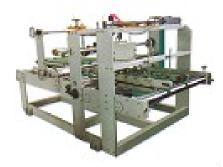
The finished product can be counted and speedchanging ctc. automatically, pile, neatly, exactly output. The speed can be adjusted, can be controlled seperately, the piling speed is 130m/min.
